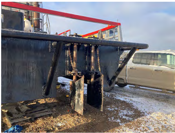
ITEM #7 Starboard Rudder Supports Renewed
