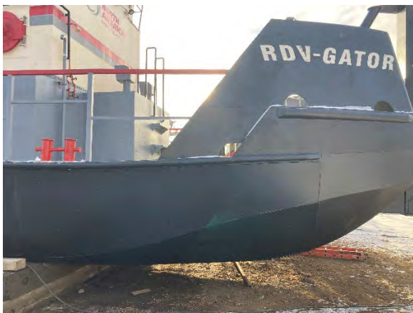
ITEM #3 Starboard Side Renewed
