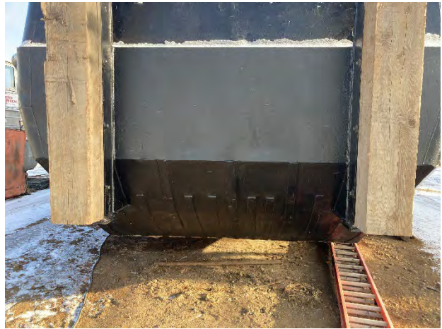
ITEM #8 Doubler Plates Removed
