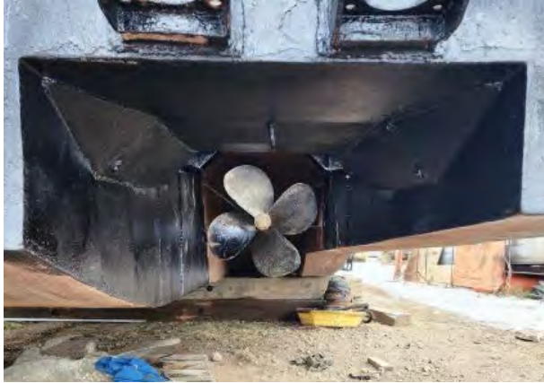
ITEM #32/33 Shafts and Props Installed Starboard
