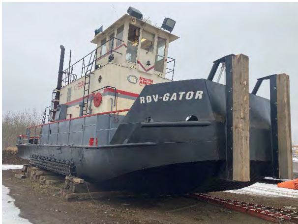
ITEM #34 Much of the vessel has been repainted top deck and hull using Carboguard 890 epoxy paint
