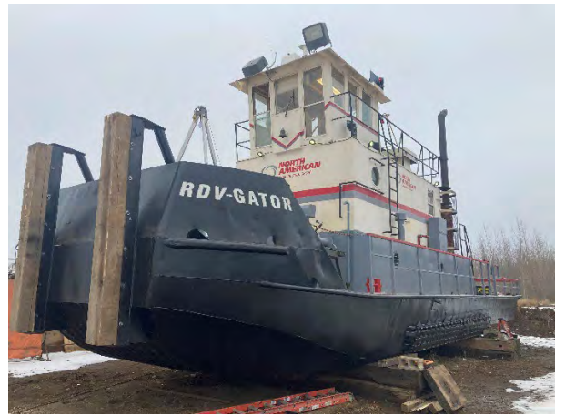
ITEM #34 Much of the vessel has been repainted top deck and hull using Carboguard 890 epoxy paint
