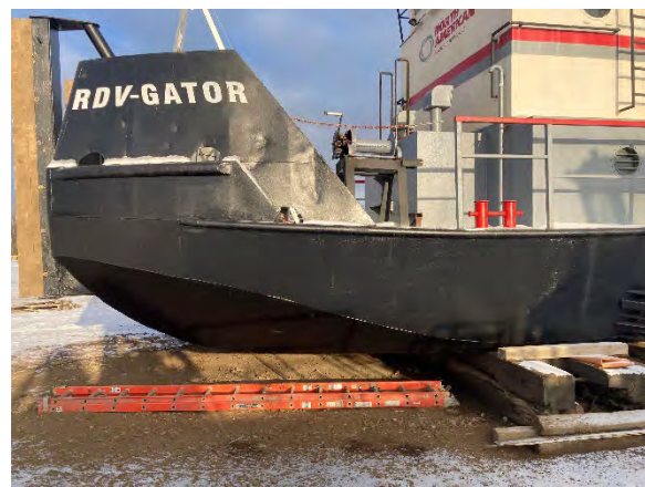
1ITEM #3 Port Side Renewed
